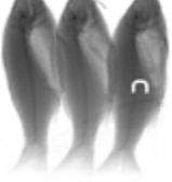
Staple identified in fish packed on foil board
