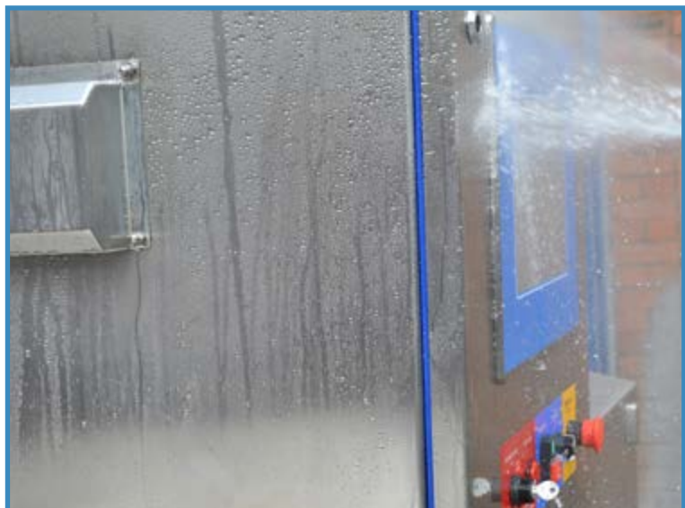
Low-pressure washdown of X-ray system
