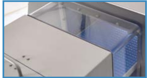
A Tunnel Guard ensures contaminated packs cannot be put on line after the metal detector
