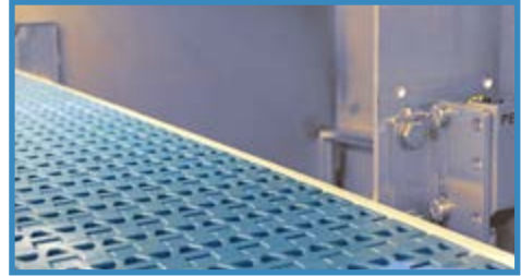
Reject Confirmation Sensor checks the pack enters the bin correctly
