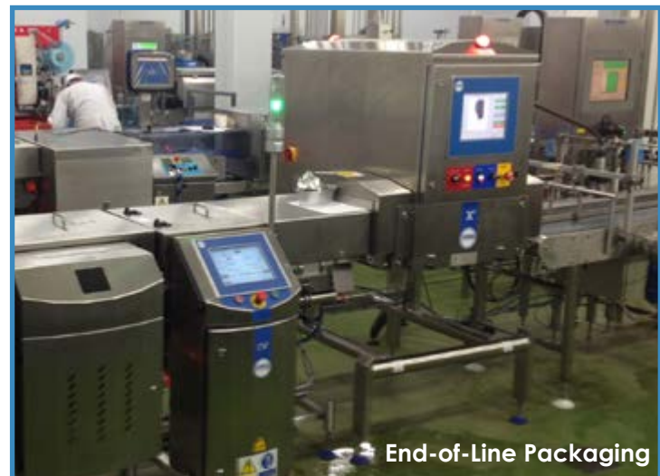
X-ray Combo systems provide detection, weighing and product integrity checks during final packaging
