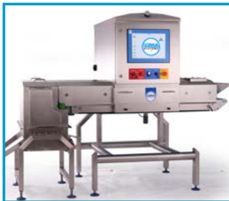
X5 Bulkflow scans fast-flowing loose product
