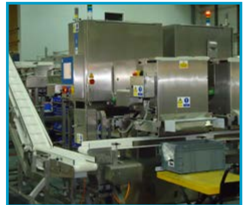
Dual X-ray system inspecting loose chicken fillets
