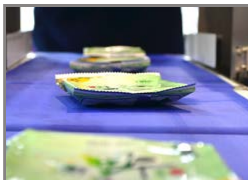
End of line checkweighing of packaged cooked meat
