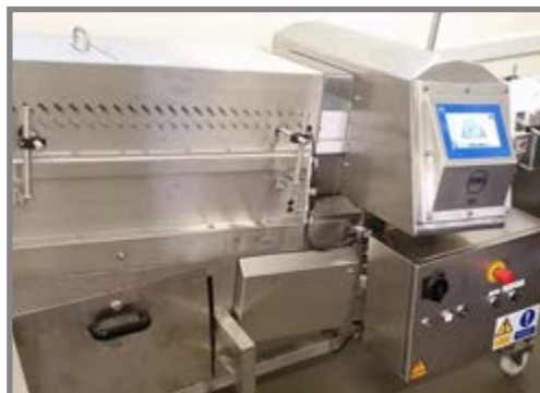
IQ4 metal detector with carriage-retract reject for packaged meat
