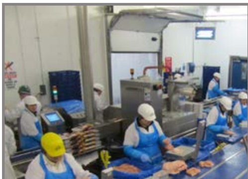
Combo system detecting and weighing processed poultry
