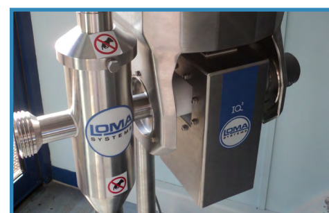
ARI Piston reject valve combined with a linker drive for integration with Handtmann vacuum fillers
