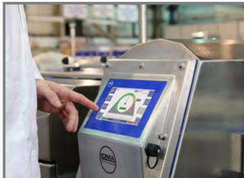
Product learn set-up on vacuum-packaged processed meat products
