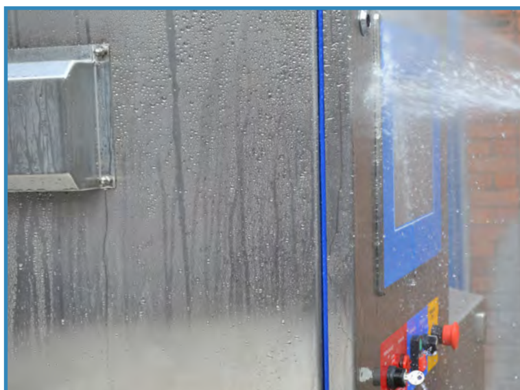
Low-pressure washdown of X-ray system
