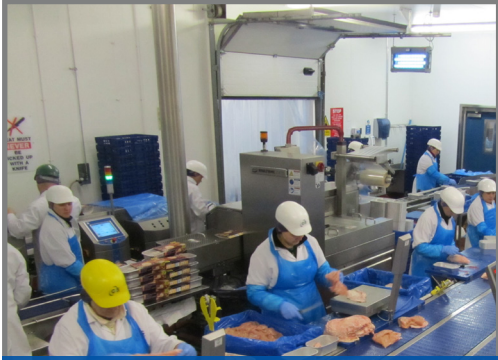
Combo system detecting and weighing processed poultry
