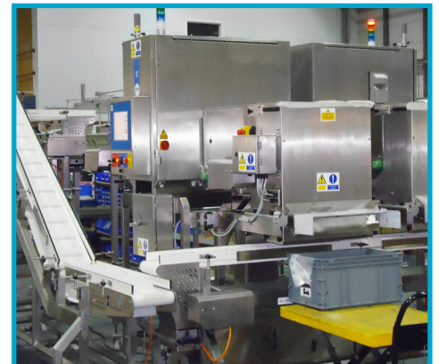
Multi X-ray system inspecting loose chicken fillets
