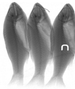
Staple identified in fish packed on foil board
