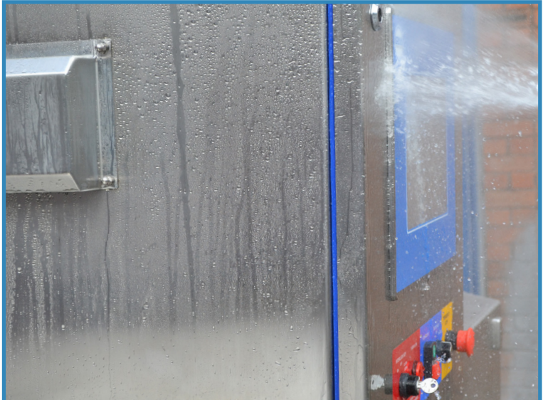
Low-pressure washdown of X-ray system
