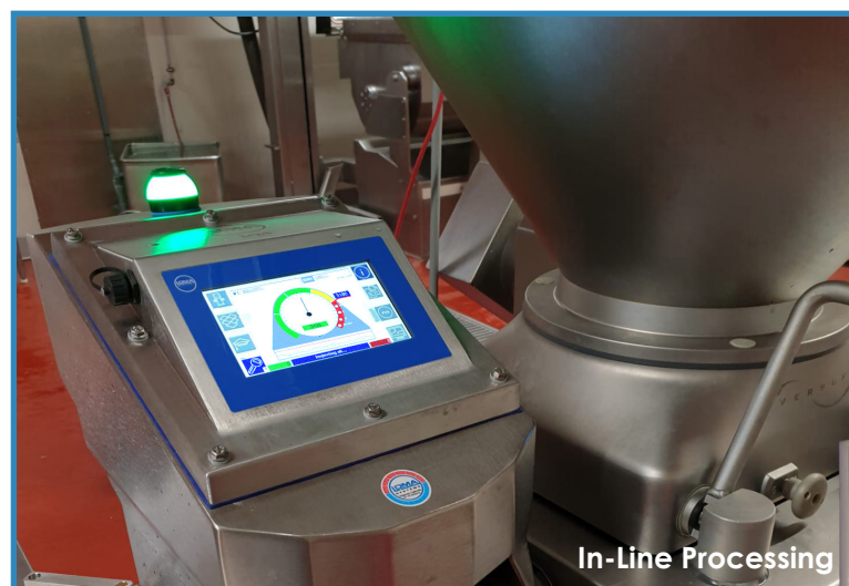
Pipeline metal detectors help protect a clipping machine from damage caused by broken metal blade fragments
