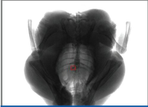
X-ray system finds stainless steel within whole chicken
