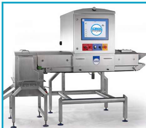
X5 Bulkflow scans fast-flowing loose product
