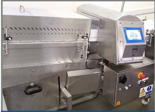
IQ4 metal detector with carriage-retract reject for packaged meat
