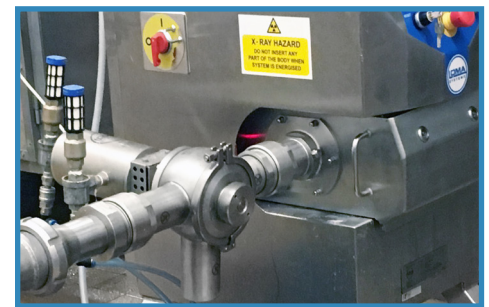
ARL Rotary reject valve used for inspecting whole muscle meat on the X5 Pipeline
