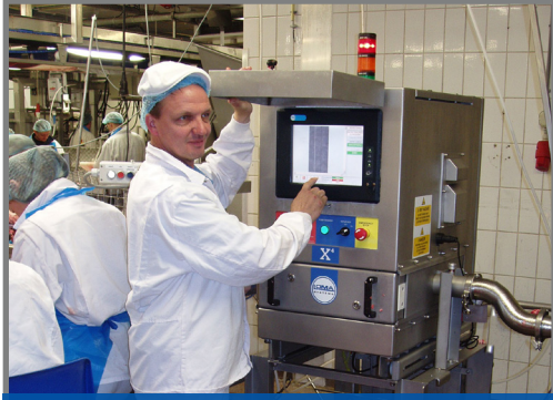
Pipeline X-ray system searches for bone, teeth and nails after mincing
