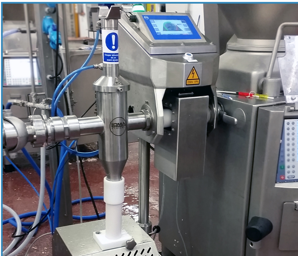
ARU Piston reject valve used for inspecting meat slurries on a metal detector
