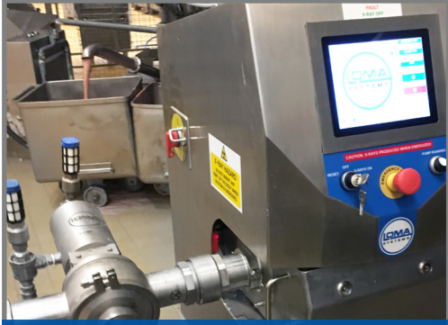
X5 Pipeline inspecting pâté meat slurries prior to filling
