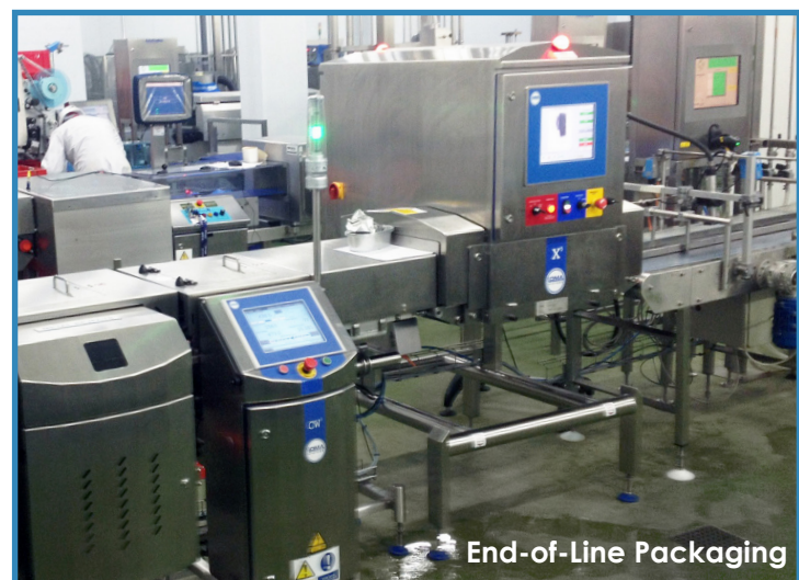
X-ray Combo systems provide detection, weighing and product integrity checks during final packaging
