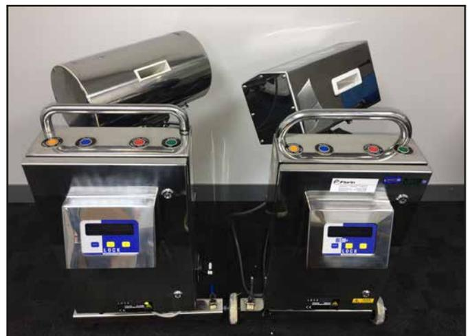
The new Metal Detector head will be mounted on your current frame and will utilize your current reject system, thus maintaining the same serial number and software versions to minimize any validation requirements. With stock of heads and mounting in our global service centers, we can offer very quick turnarounds on this program.
