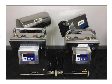
The new Metal Detector head will be mounted on your current frame and will utilize your current reject system, thus maintaining the same serial number and software versions to minimize any validation requirements. With stock of heads and mounting in our global service centers, we can offer very quick turnarounds on this program.
