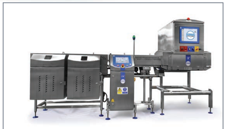
X5 Space Saver X-ray / CW3 Combination System
