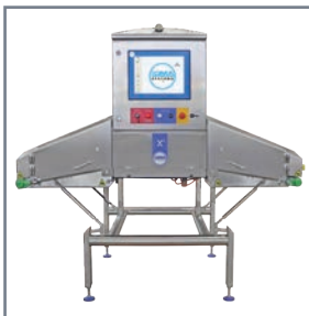
X5 Pack Curtainless is designed for lightweight, unsealed or dry unpackaged food products
