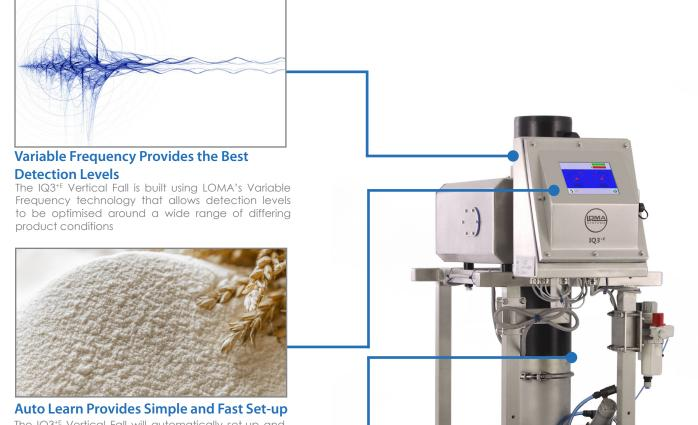
The IQ3<sup>+E</sup> Vertical Fall will automatically set-up and store up to 200 different presets, calibrating for product effect and loose material as the product passes through the system.
