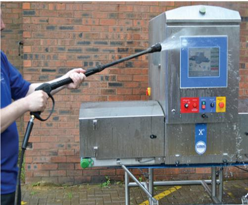
The Loma Systems X5 x-ray inspection system is designed to withstand the rigors of harsh washdown environments.
