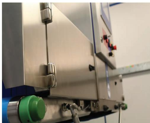
The new quick release belt feature enables you to easily pull out the conveyor belt for easy cleaning, maintaining hygiene in any production environment.
