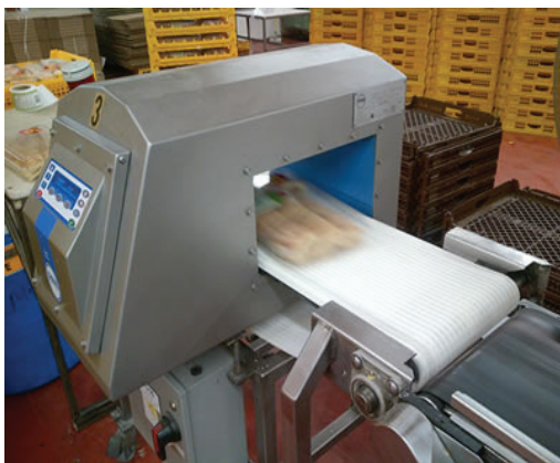
Companies rely on the speed and efficiency of the Loma Systems IQ3 metal detector as part of their quality control program.
