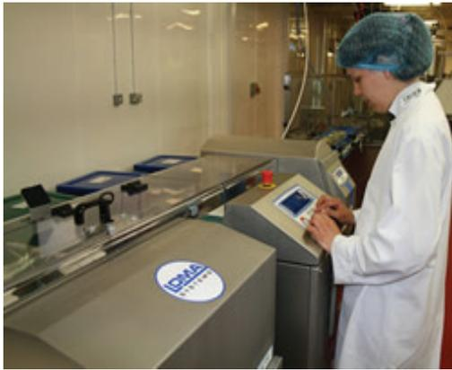
To save space, companies often turn to combination systems, that incorporate both checkweighing and metal detection.
